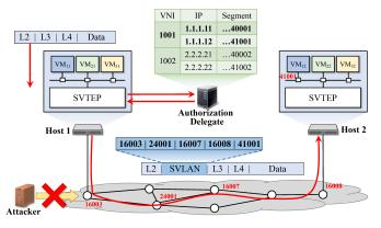
Fig. 3: Only authorized senders can retrieve valid path segments and forward packets to the receiver.
