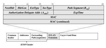
Fig. 4: The header format of the SVLAN extension.
